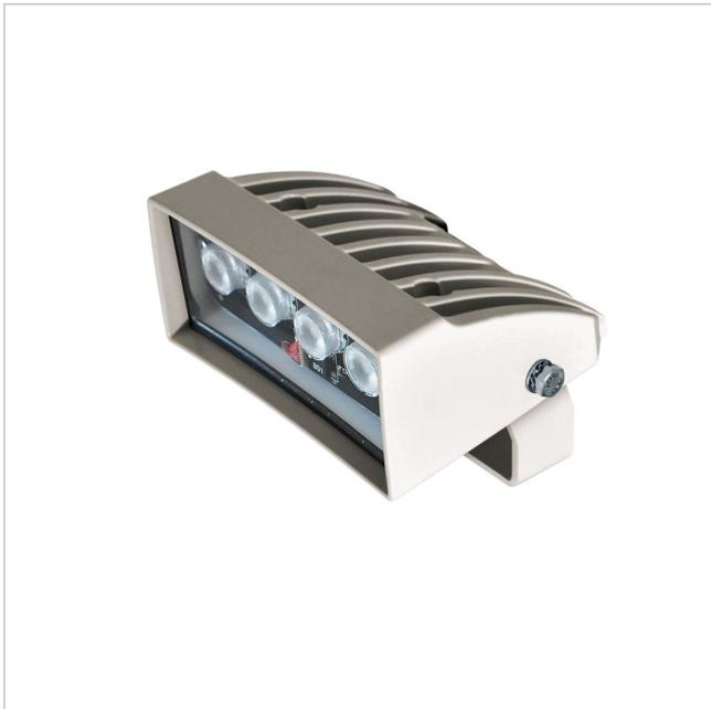
LED Infrarot Scheinwerfer, 850nm, 30°, 84m, IP66/67, 12-24VDC/24VAC
