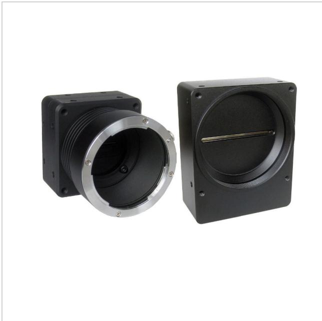
Dual Line, S/W Zeilenkamera, 8k, CMOS, 7µm, 80kHz, Camera Link, M72-Mount
