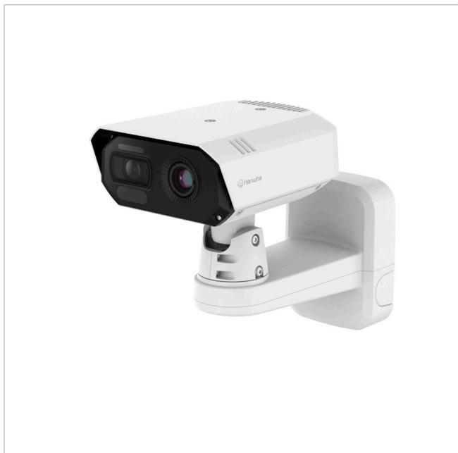
Bi-Spektrum KI-Wärmebildkamera, VGA 9,1mm 8fps, 8M MVF 4,4-9,3mm 30fps, IP66/67, IK10, PoE+, 12VDC
