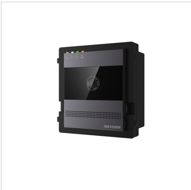
2-Draht Türstation, 2MP, WDR, H.264, Fisheye, 48VDC, IP65, IK08
