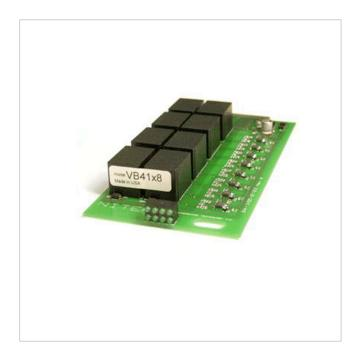
8 channel Passive Transceiver UTP Card, up to 225 m
