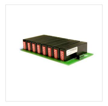
8 channel Active Receiver UTP Card, 900m, up to 1800m with active transmitters
