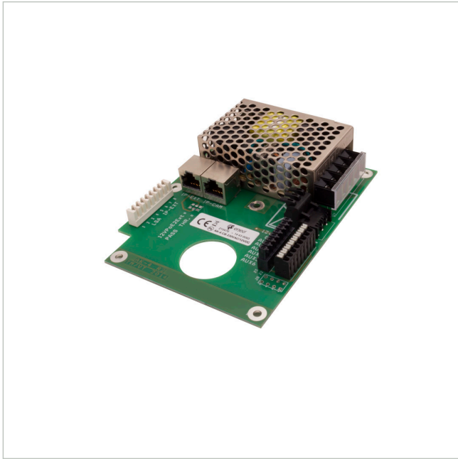
Connection board with 12V power supply
